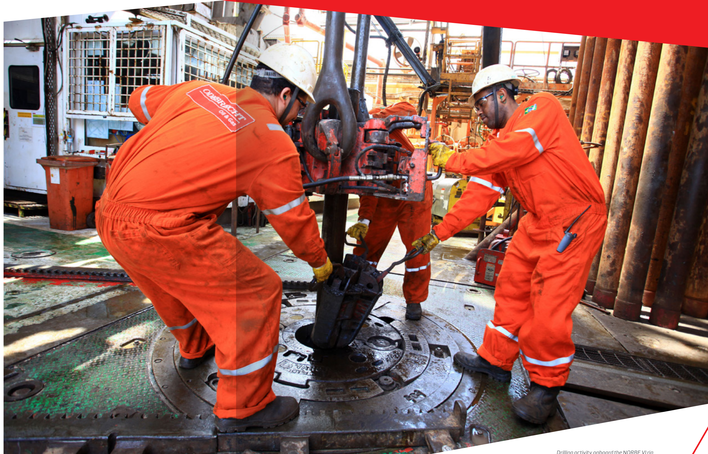
Drilling activity onboard the NORBE VI rig
